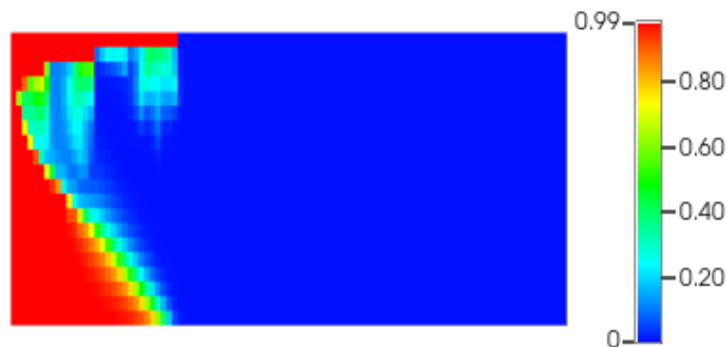
Figure 2. CO 2 spatial distribution for zero water salinity (pure water)
