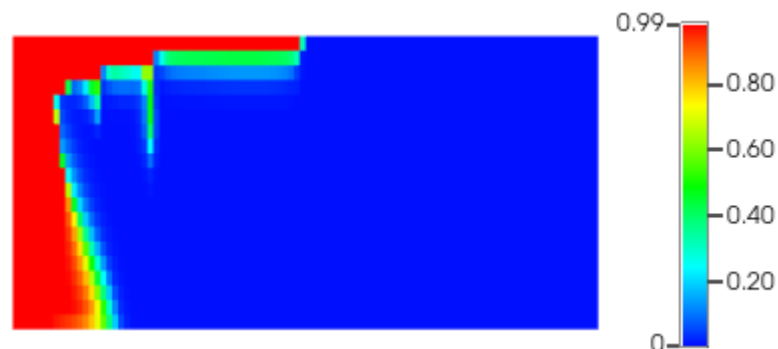
Figure 8. CO 2 spatial distribution for 300000ppm water salinity level
