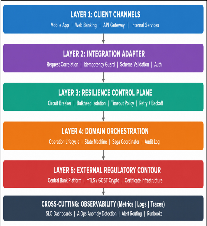
Figure 2. Layered Architecture of a Critical Banking Integration Circuit with Embedded Resilience and Observability Controls (author-developed based on [6, 7, 10, 12, 13]).
